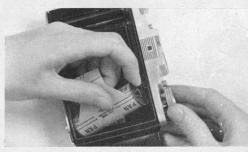
tapered end of the backing paper and seal it with the gummed strip. Keep the film out of bright light until you hand it to a Kodak dealer for developing and printing.
