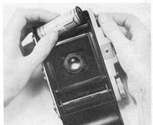
Break the paper seal, and draw the backing paper across to the empty spool. Thread the tapered end as far as it will go through the longer of the two slots in the spool until it protrudes through the other side. Centre the paper carefully on the spool.
